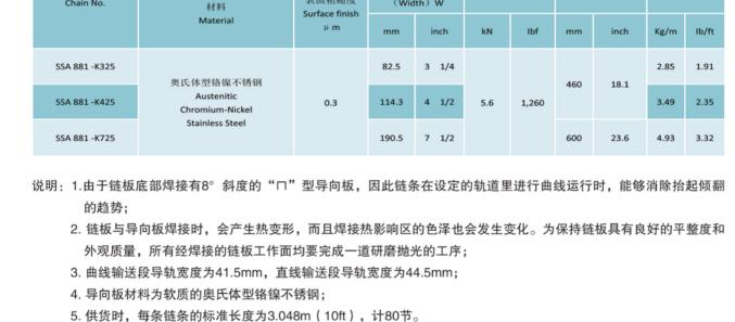
plate that has been welded needs to be polished by grinding. 3. The width of the track in the curve conveying section is 41.5mm, and the one of the track in the straight conveying 4. The material of bevel shoe is Soft Austenitic Chromium-Nickel Stainless Steel.
